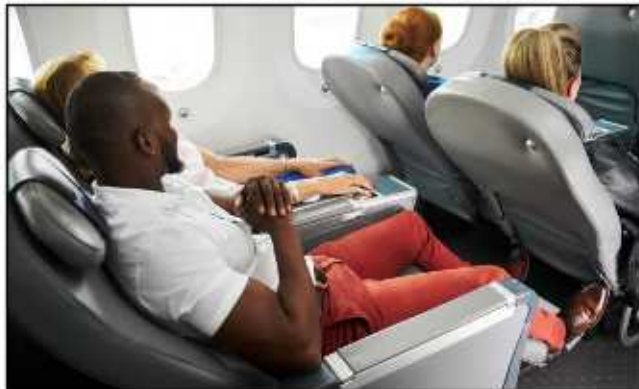
The 43-inch pitch for Premium class on Norse Atlantic is more generous than the usual 38-inch pitch found on global network airlines. Image: Norse Atlantic
