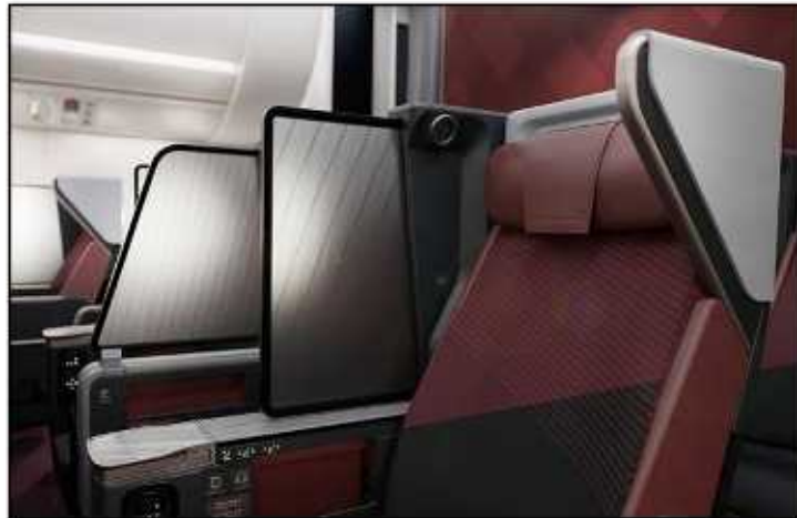
The Japan Airlines premium economy seat on A350 aircraft features a fixed shell which preserves space for the person behind you when the seat reclines.
